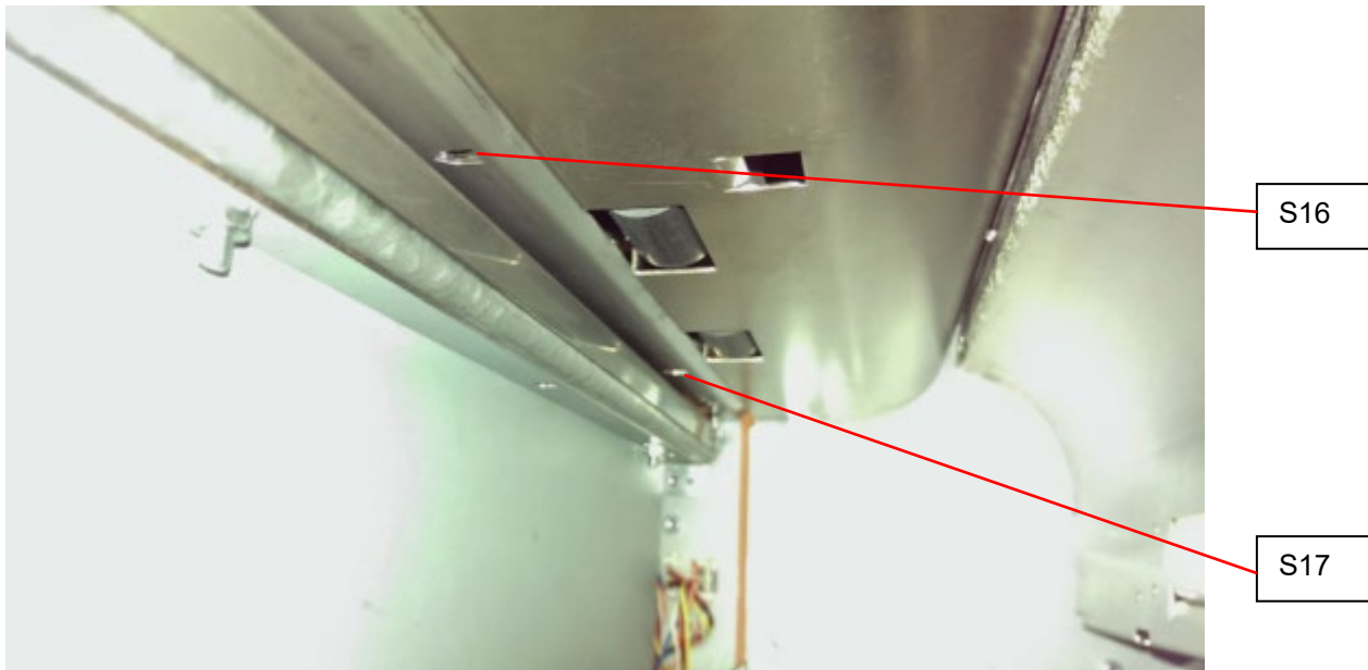
Sensors S16 and S17 are on Backgage Sensor Board.
