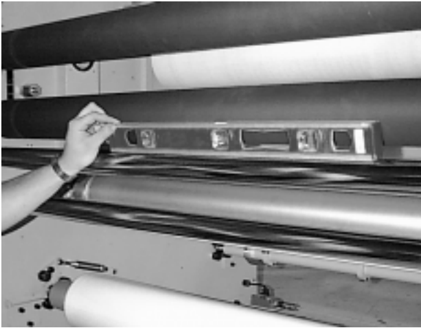
Figure 2-8: Leveling Side to Side
