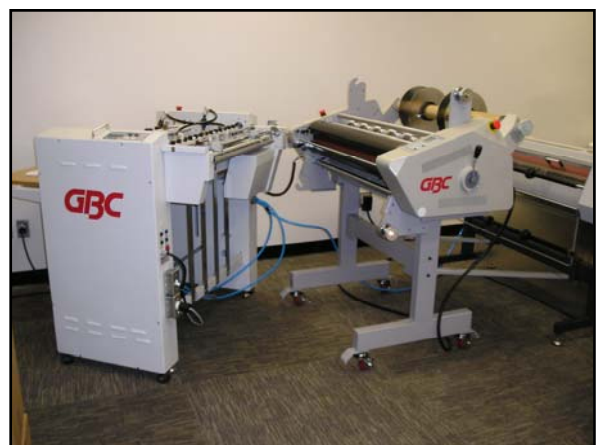
Swing out feeder to load bottom film roll.
